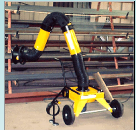
Local Exhaust Ventilation
