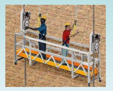
This working platform is using the permanent hoist machine and roping, and requires the installation of the governor. The governor rope must be attached to the safety releasing arm and tested to ensure that the safety is operational.
