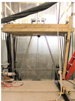
False car frame and platform
