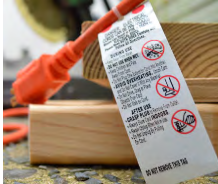
Listing label attached to an extension cord
