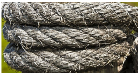
Figure 2 - Poor quality manila rope
